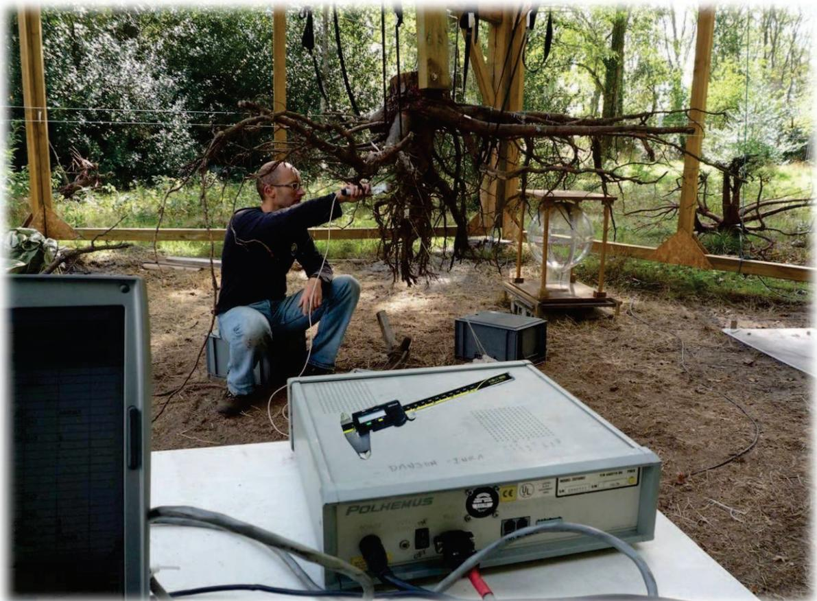
*Digitizing of a root system at the laboratory of Pierroton. Spatial coordinates, topology of the origin of all root axes and the end of all root segments, were measured
